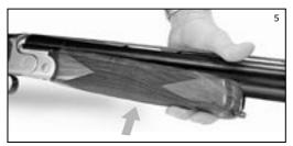
Only then is the fore-end secured and the barrels safe to open.
