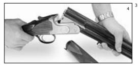
Make sure this locking block engages in the receiver then move the top lever to the right and close the breech.
