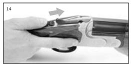
Take the shotgun off safe by pushing the safety forward with the thumb of the shooting hand (figure 14).
